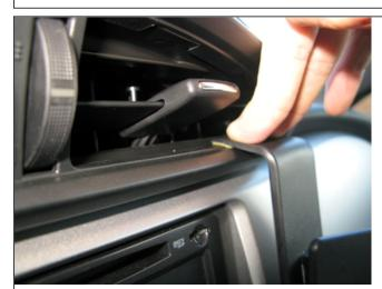
3. Press downward on top of the  $\mbox{ProClip}$  so the angled edge goes all the way into the gap.
