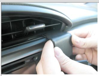
2. Pull the upper part of the ProClip upward and hook the angled edge into the gap between the air vent and the surrounding frame inside the lower part of the air vent
