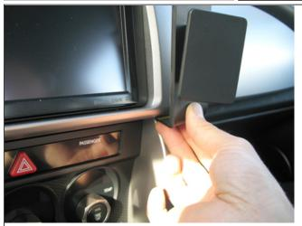
1. Use the enclosed alcohol pad to clean the area where the ProClip is to be installed. Peel off the adhesive tape covers on the ProClip. Press the angled edge on the lower part of the ProClip into the gap between the upper section of the dashboard and the frame surronding the control panel.
